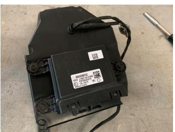
On passenger side remove(4) Phillips screws
