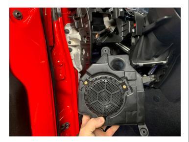
• Remove the module from the OEM enclosure
