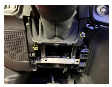
• Clip the instrument panel shroud into place
