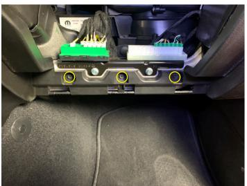
Looking in the glovebox cavity up high, remove two 13mm bolts securing the back of the passenger side airbag
