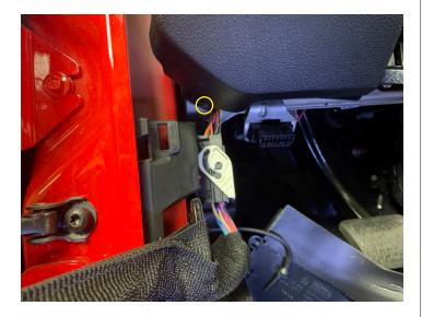
• Remove (2) Phillips screws near steering column
