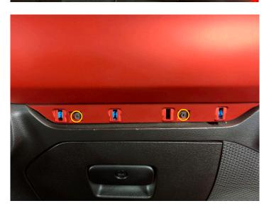
Remove glove box by opening and lifting the upper tab and removing the latch on the left side
