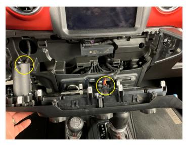
• Connect the wiring and clip the climate control panel into place
