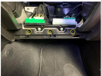
Install glovebox by installing bottom hinge and pivoting up. (Also install left side gear arm)
