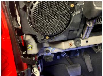
• Remove (3) Phillips screws securing the speaker enclosure
