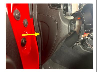
• Clip the steering column shroud into place
