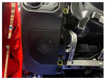
Remove (2) Phillips screws on the top of the left dash then unclip and disconnect wiring on back of light switch to remove panel from vehicle
