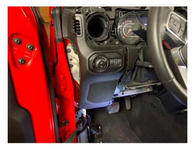
• Install (2) Phillips screws on the top of the left dash
