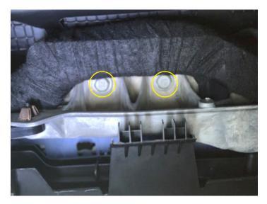
• Install (3) Phillips screws at bottom of glovebox opening
