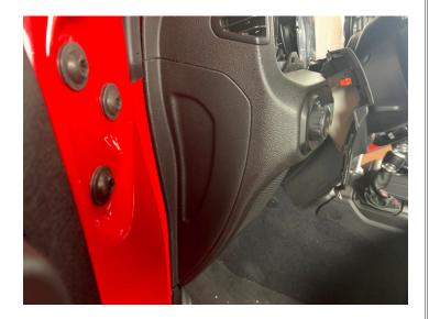
• Remove (5) Phillips screws that are exposed
