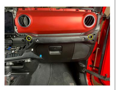
• Slide ears on cover into slot and snap grab handle cover into place
