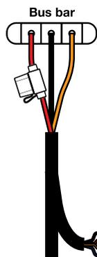
If you are connecting the amplifier into an existing Stage 2 system - either MBQR-STG2-RAD-2 or MBQR-STG2-RC-1, simply plug in the unused power/ground connector of the the mono amplifier into the Stage 2 harness. At the same time, if you have (or will later install) optional illuminated MB Quart SR1-120RGB LED light rings for the 8" compression horn front or rear speakers, connect the red/black wires as well. See Figure 9-1 for the connection diagram.
