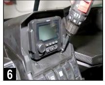
Remove four T-25 screws securing the source unit housing to the center of the dash. Two in front, two in back near master brake cylinder.
