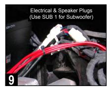
Connect the electrical and speaker plugs for each amplifier as labeled\*. Tie up excess wiring to factory wires and avoid any moving parts.
