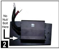
Attach 400.1 amplifier to mounting plate with included hardware as indicated. Use only three nuts/bolts due to tube frame clearance.
