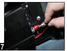
Connect the RCA audio cable extension to Sub Amp 2 inputs. Position of right or left RCA plugs does not matter because the output signal is mono.
