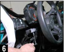
Remove two T-30 screws holding the gauge cluster with a 10mm socket (below) and T-30 driver (above). Set gauge cluster aside when done.
