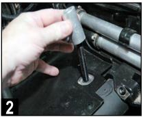
Remove the factory-supplied aluminum spacers from rear bolts of seat mounts\*. Replace with supplied MB Quart spacers for bracket tolerance.
