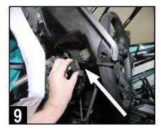
Pull panel\* carefully to access switches and unplug them to fully remove driver's side panel. Set aside as with passenger dash panel for later reuse.
