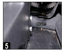
Attach front right side mounting brackets to the subwoofer enclosure using two 1/2" bolts and a lock washer on each.
