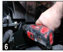
Drill mounting holes in the marked locations using a 1/8" drill bit. You may wish to remove the amp plate before drilling to avoid scratch marks.
