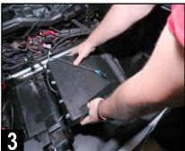
Load subwoofer enclosure into under passenger seat position by angling the front under the support bar for clearance of the brake line and to sit level.
