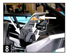
Remove two T-30 screws on the side edge of the panel. Next, remove two remaining T-30 screws behind gauge cluster area as indicated.
