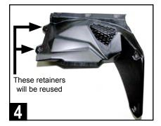
Gently remove passenger side speaker panel and set aside. The center push pin retainer clips will eventually need to be transfered to the new panel.
