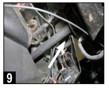
Remove one additional hidden push pin under the driver's side dash, between the steering wheel and console, just forward of the tubular chassis support.
