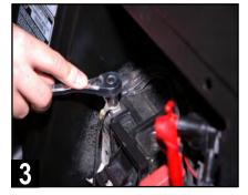
Repeat seat removal on front passenger's side. Once passenger seat near battery is removed, disconnect (black) negative battery cable by removing a 10mm bolt and set the negative cable aside.
