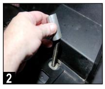
Remove the factory-supplied aluminum spacers from rear bolts of seat mounts\*. Replace with supplied MB Quart spacers for bracket tolerance.
