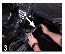
Remove front of center console side panel on passenger's side (footwell area) using a pry tool to gently release the pressurefit clips.
