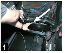
Remove driver's side console side panel using a pry tool from the top to gently release the pressure-fit clips.
