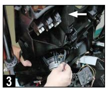
Connect driver's side speaker to white speaker wiring near the amplifier harness area. Red/black wires are for optional illuminated speaker rings.
