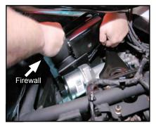
From the top side, place amplifier plate in the intended location behind silver brake booster against the driver's side firewall for test fitting.
