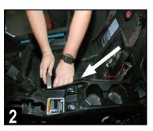
Remove passenger's side console side panel using a pry tool from the top to gently release the pressure-fit clips.
