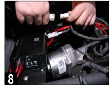
Connect the speaker (Sub 2) and power harness connectors as shown.
