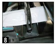
Gently remove the four visible push pin clips with a panel removal tool or special panel clip pliers (not needle nose) as shown.
