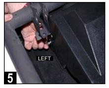
Attach front left side mounting brackets to the subwoofer enclosure using two 1/2" bolts and a lock washer on each.
