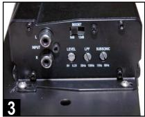
Next, make initial LEVEL, LPF crossover and SUBSONIC filter settings as indicated on the 400.1 amplifier (Sub Amp 2).
