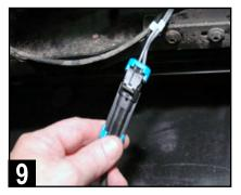
Connect the enclosure's wiring pigtail to the connector at the side of the console labeled "Sub 1." If tucked away, side of console may need removal.
