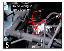
Route power, speaker wiring and RCA extension to amplifier location (near frame tubes). Place mounting clamps in initial locations as shown.
