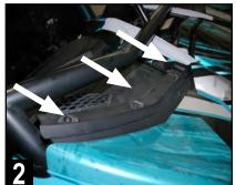
Remove three T-30 screws from the top edge of the passenger's side dash where the hood line meets the dash as indicated.
