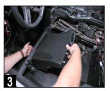
Load subwoofer enclosure into under seat position by angling the front under the support bar for clearance of the brake line and to sit level.
