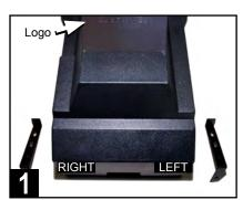
Identify front enclosure brackets. Orientation is referenced to the logo. Left and right are stamped "L" and "R" on the bracket and enclosure.
