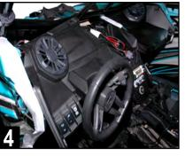
Set panel temporarily in place without attaching any hardware or clips. Do not yet plug in switches in case subwoofer amplifier adjustments are needed.
