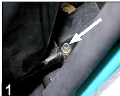
Slide driver's seat forward and remove two 18mm bolts securing the rear of the seat frame. If the vehicle has factory-installed seats, you can also access these bolts by flipping up the seat cushion (a socket extension is required).
