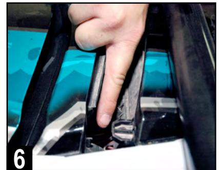
6 Next, remove two additional T-30 screws located beneath the forward edge of the top center plastic cover location, just forward of fuse box.
