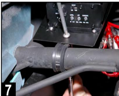
Place amplifier & plate into its location. Attach the supplied Phillips screws and 7/16" nuts through the clamp holes and tighten until amplifier is secure.
