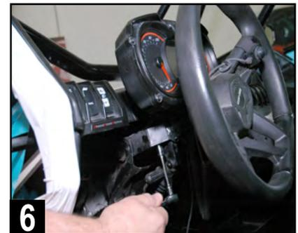
6 Remove two T-30 screws holding the gauge cluster with a 10mm socket (below) and T-30 driver (above). Set gauge cluster aside when done.
