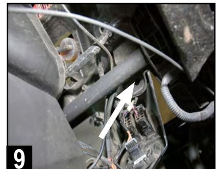
9 Remove one additional hidden push pin under the driver's side dash, between the steering wheel and console, just forward of the tubular chassis support.
