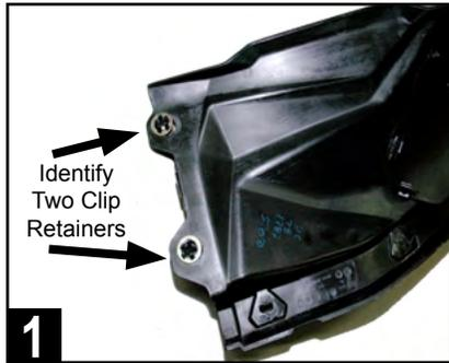
1 Locate the factory front left and right speaker panels and identify two mounting clip retainers and washers that need to be removed on each.
