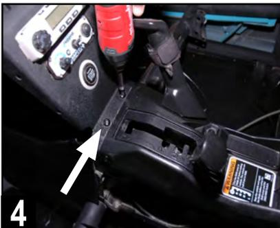
4 Move gear selector all the way back (away from the dash). Remove two T-30 screws from the area just forward of the gear selector when in park.
