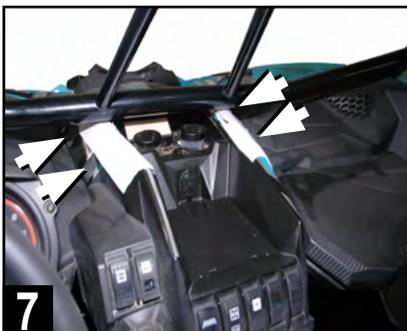
7 Identify four visible push pin clips on the outer edges of the center pocket. These secure the flanges of the left and right side dash speaker panels.
