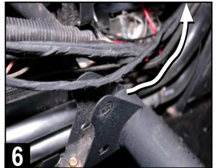
Route your wiring upward behind the center dash as indicated where the panel was removed. Secure with zip ties to factory wiring.
