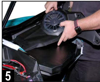
5 Begin to set passenger side speaker panel in place by loading the edge nearest the center with the clip retainers into position as shown.
