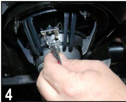
4 Connect passenger side speaker to your installed speaker wire. Crimp connectors are needed to mate with speaker terminals.
