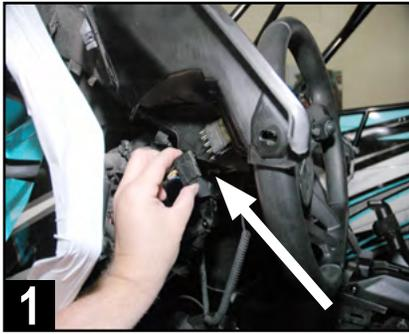
Plug in all switch wiring on back of the driver side front speaker panel. Test switch functions to ensure they are correctly connected.
