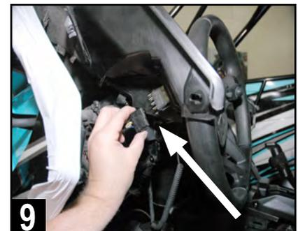
9 Pull panel\* carefully to access switches and unplug them to fully remove driver's side panel. Set aside as with passenger dash panel for later reuse.
