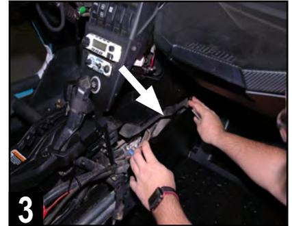
3 Remove front of center console side panel on passenger's side (footwell area) using a pry tool to gently release the pressure-fit clips.
