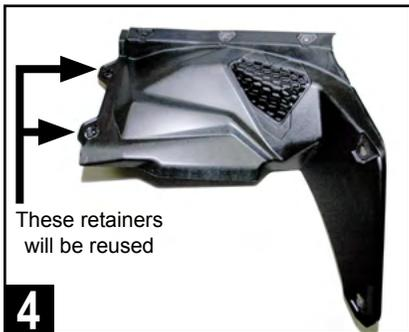
4 Gently remove passenger side speaker panel and set aside. The center push pin retainer clips will eventually need to be transferred to the new panel.
