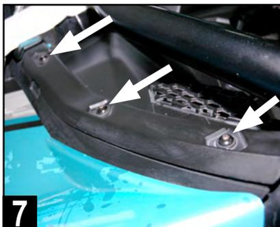
7 Remove three T-30 screws from the top edge of the driver's side dash where the hood line meets the dash as indicated.
