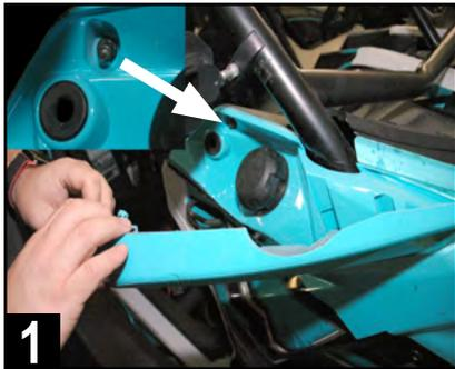
1 Remove gas filler access door on passenger side. Note above the grommet for the retainer clip, there is a 10mm nut attaching a mounting screw.
