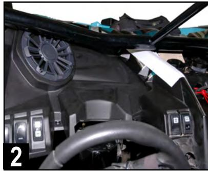
Place driver side speaker panel into its final position\*. Check fit so that all open hardware and clip holes are aligned properly.
