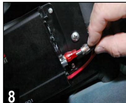
Connect the RCA audio cable from source unit to left and right channel amplifier inputs. Be sure to double check left is left and right is right (channel).
