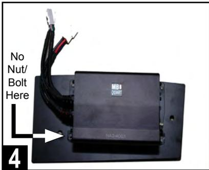
Attach the 400.2 amplifier to mounting plate with included hardware as indicated. Use only three nuts/bolts due to chassis tube frame clearance.
