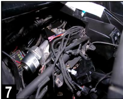
Route your wiring up to steering column support bar area. This allows space to work for likely amplifier and source unit locations.
