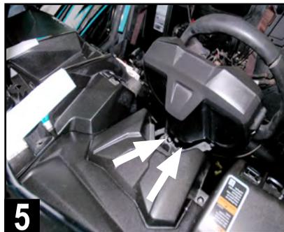
5 Drop steering wheel position to access two T-30 gauge cluster screws. Cluster removal helps removal of the panel and access for amplifier installation.
