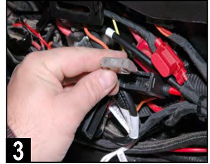
Remove the fuse from the main fuse holder you've installed so the power wiring is not live while routing through the vehicle.
