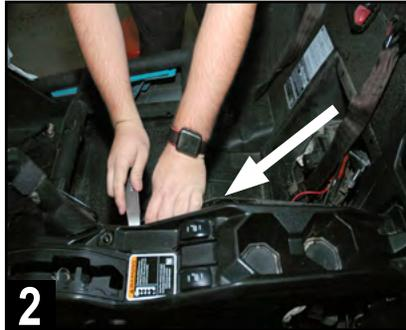
2 Remove passenger's side console side panel using a pry tool from the top to gently release the pressure-fit clips.
