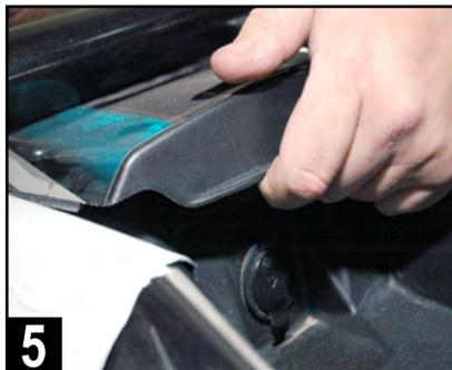
5 Remove top center plastic cover above dash pocket by pushing up on the front pocket edge above the lighter socket, then pulling toward you.
