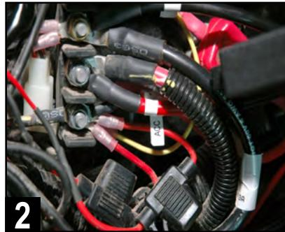
Connect your Ground, Battery and Ignition wires to the bus bar locations. Ensure there is a fuse holder on the main +12 volt battery connection.
