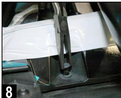
8 Gently remove the four visible push pin clips with a panel removal tool or special panel clip pliers (not needle nose) as shown.
