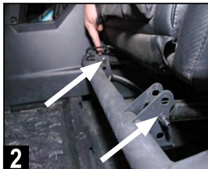
Slide driver's seat back to access front 13mm through-bolts and nuts. Using a socket and box wrench, remove inner and outer front seat hardware. Unplug seat belt sensor. Remove front driver's seat and set aside with all hardware.
