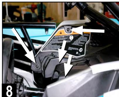
8 Remove two T-30 screws on the side edge of the panel. Next, remove two remaining T-30 screws behind gauge cluster area as indicated.
