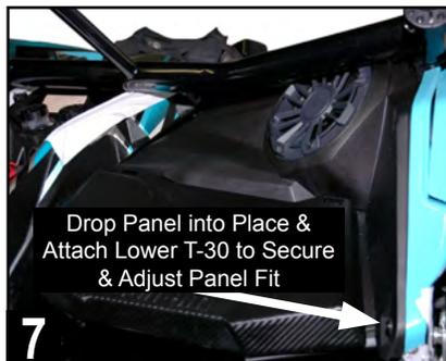
7 Next, drop the speaker edge of panel into place\*. Attach lowest T-30 screw into place to allow check of final panel fit and to ensure all clip holes align.
