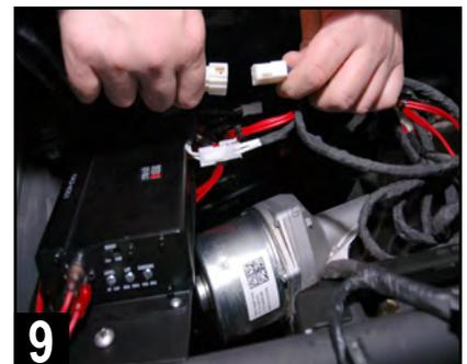
Connect the 4-pin speaker and 3-pin power wire harness connectors as shown. Zip tie wiring to void any moving parts, moisture or heat sources.
