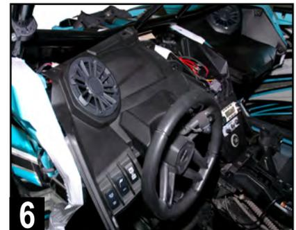
6 Set panel temporarily in place without attaching any hardware or clips. Do not yet plug in switches in case amplifier adjustments are needed.
