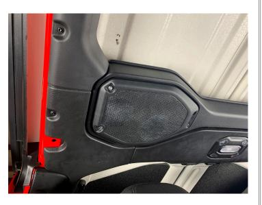
Remove and disconnect (4) T30 Torx screws from the port and (5) T20 Torx screws from both speakers
